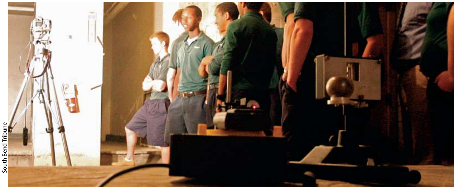
A mirror attached to the apparatus in the foreground reflects a laser beam onto the wall in the background. The digital camera on the left takes pictures of the reflected laser beam.
